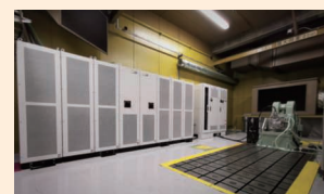
EVs motor and battery emulator for evaluation
