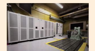
EVs motor and battery emulator for evaluation
